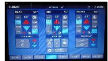
Figure 4-7: Heat Pump Controls
