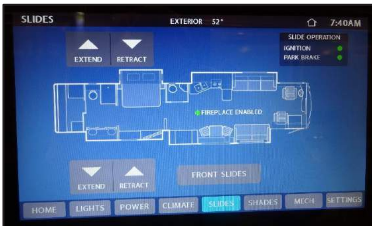
Figure 10-1: Slide-Out Screen on the Spyder Controls System
