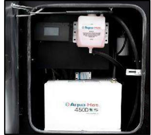
Figure 13-18: Aqua-Hot Surge Tank
