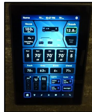
Figure 0-6: Spider Controls System Switch
