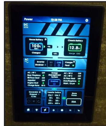
Figure 0-12: Energy Management System
