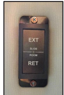
Figure 10-2: Front Slide-Out Switch
