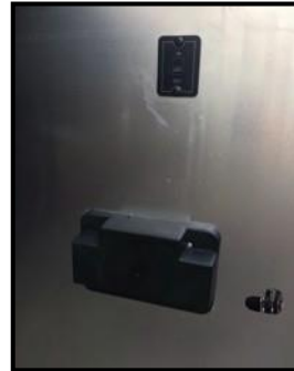
Figure 11-3: Electric Slide Tray Switch on Cargo Door
