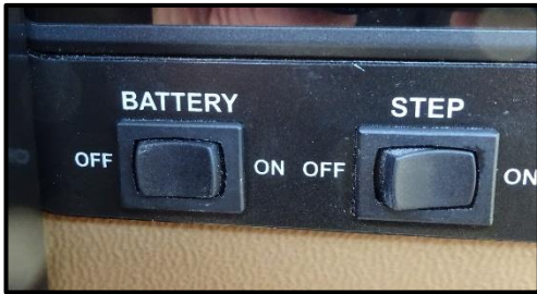
Figure 9-6: 12 VDC Disconnect Switch
