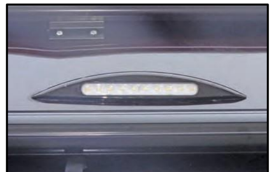
Figure 11-4: Exterior Security Light
