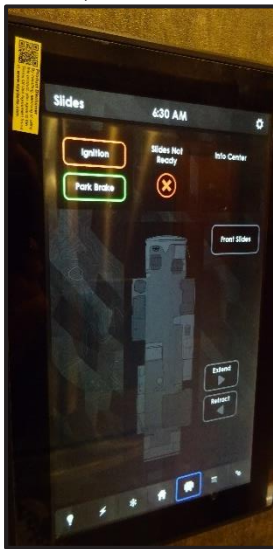
Figure 10-1: Slide-Out Screen on the Spyder Controls System
