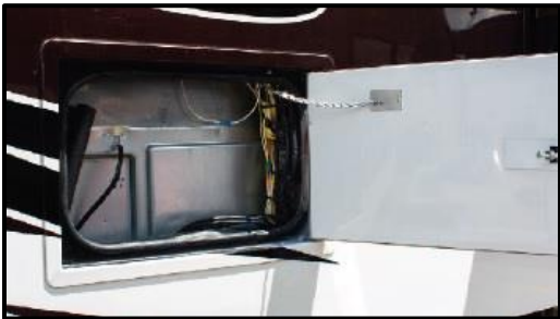
Figure 11-9: Outside Refrigerator Access
