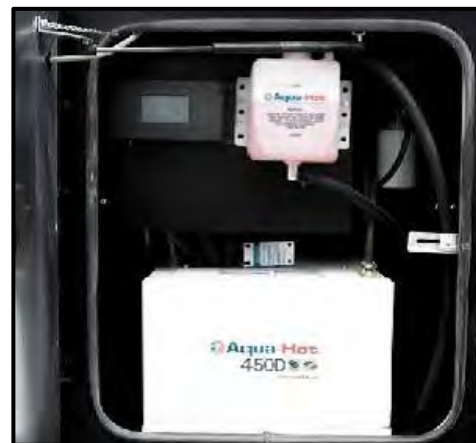
Figure 13-18: Aqua-Hot Surge Tank
