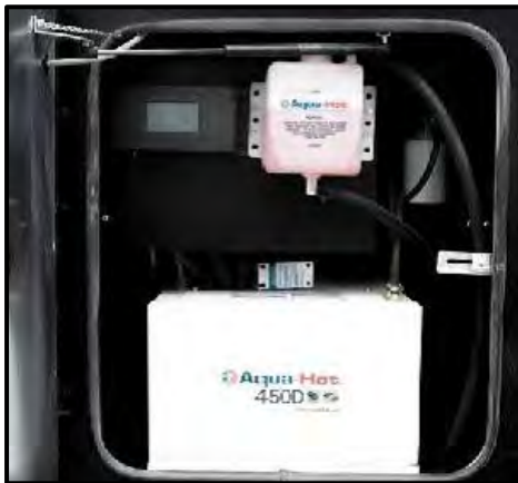
Figure 4-2: Aqua-Hot Surge Tank
