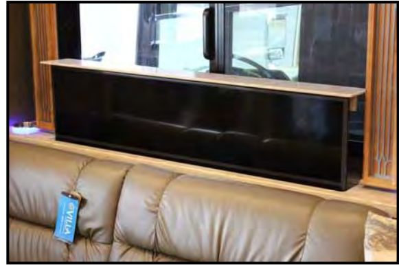
Figure 6-4: Television Lift (Lifting)
