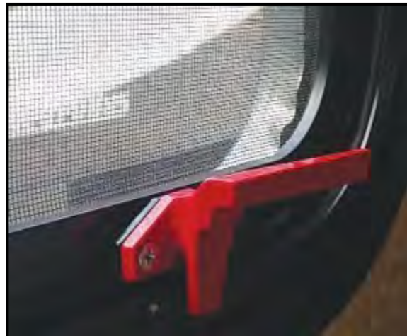
Figure 2-6: Emergency Exit Latch
