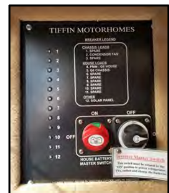
Figure 9-4: House Battery Disconnect Panel Switch
