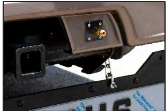
Figure 2-7: Towing Hitch & Tow Brake Air Outlet
