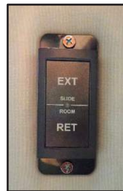
Figure 10-2: Front Slide-Out Switch
