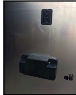
Figure 11-4: Electric Slide Tray Switch on Cargo Door
