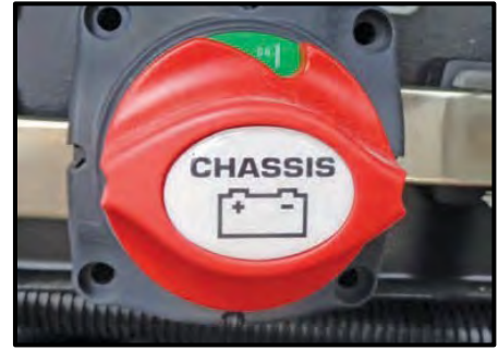
Figure 9-6: Engine Battery Disconnect Panel Switch
