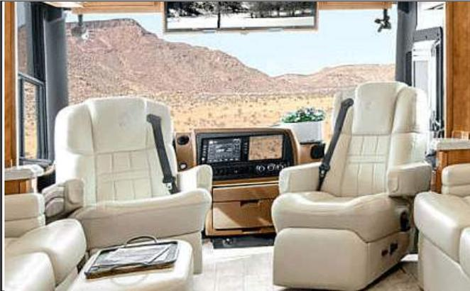
Figure 7-7: Both the driver's and passengers chairs swivel to face the living area of the coach.
