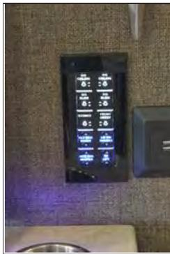
Figure 6-7: Television lift control panel located in the living room slide-out box
