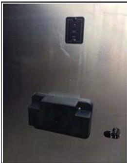
Figure 11-4: Electric Slide Tray Switch on cargo door
