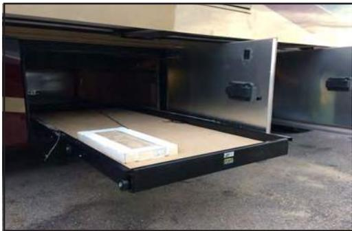
Figure 11-3: Extended Electric Cargo Tray
