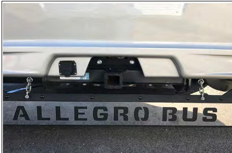
Figure 2-8: Towing hitch
