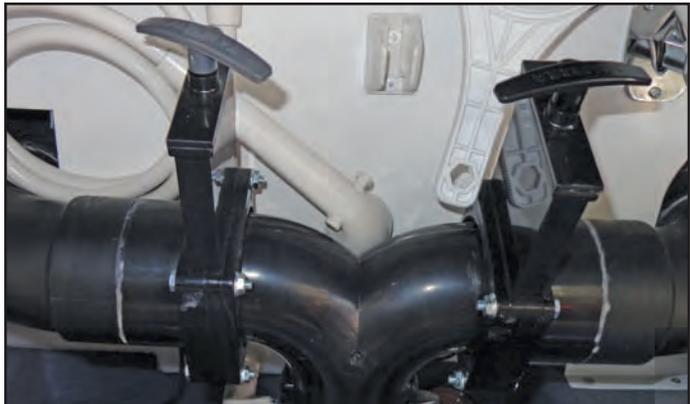
Figure 13-11 : Sanitation Coupling
