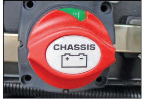
Figure 9-5: Engine battery disconnect panel switch
