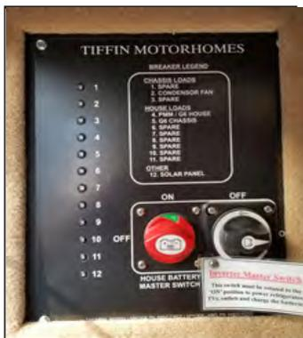
Figure 9-4: House battery disconnect panel switch
