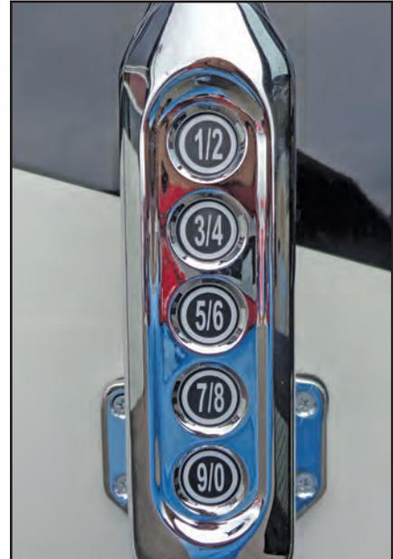
Figure 14-7: Allegro Bus keyless lock and handle
