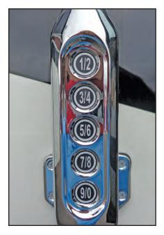
Figure 14-4: Allegro Bus keyless lock and handle
