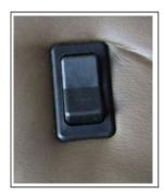
Figure 10-2: Slide-out switch on passenger and driver seat
