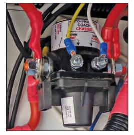
Figure 9-6: 12 VDC disconnect switch
