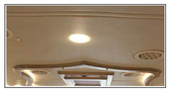
The ceiling (Figure 12-4) in the Allegro Bus motorhome is covered with a padded vinyl headliner which can be easily cleaned with a damp, soft cloth and a mild detergent.
