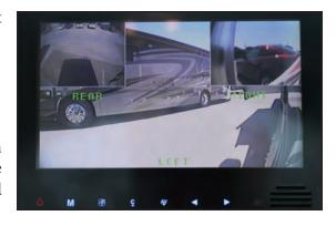
Figure 15-2: Side-mount camera monitor
