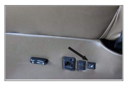
Figure 7-8: Heated Seat Switch
