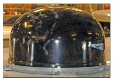
Figure 6-2: The dome satellite on top of the motorhome can be raised allowing easy access to change switches to a new satellite provider.
