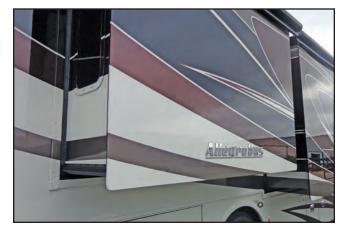
Figure 10-3: Typical slide-out fully extended
