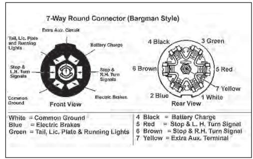
Figure 9-17: Seven-Pin towing connector
