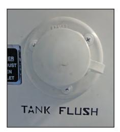
This vehicle may be equipped with a flushing system for the black-water holding tank. When draining your sewer tank, attach a water hose to the sewer spray connection. After the tank is drained, leave the gate valve "open" and open the water valve to allow water to spray inside the black-water tank. This will clean the inside of the tank of any debris that may be left inside the tank. After this procedure is done, disconnect the freshwater hose and close the gate valve.
