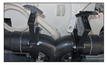
Figure 13-10:: Sanitation Coupling
