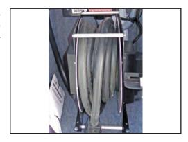
Figure 9-15: Electrical power cord reel
