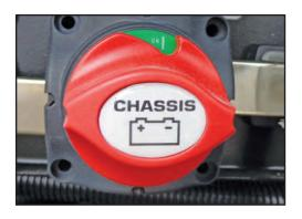
Figure 9-5: Engine battery disconnect panel switch
