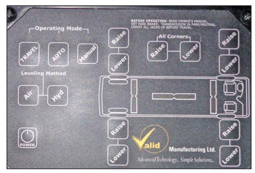
Figure 15-5: Optional air leveling system control panel
