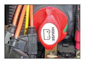
Figure 9-4: House battery disconnect panel switch
