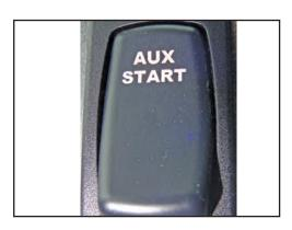
Figure 9-2: Auxiliary start switch
