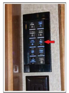
Figure 7-10 Touchpad for Power Smart Bed.
