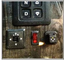
Figure 11-8: Mirror adjustment controls
