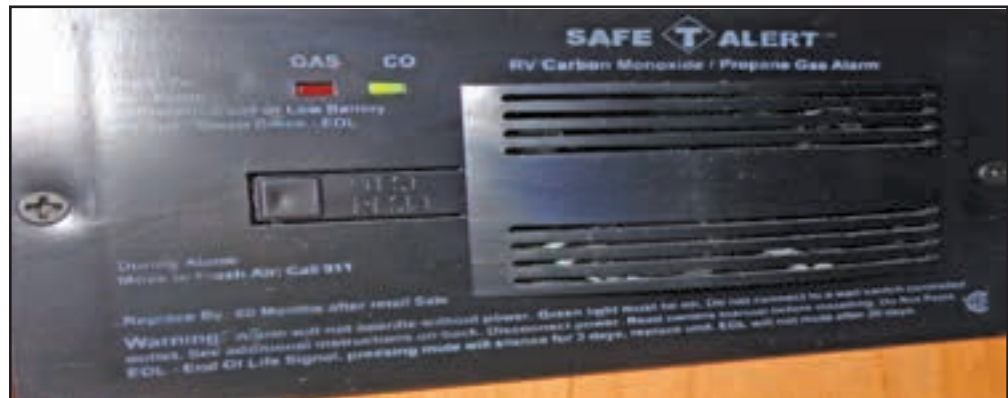
Figure 2-6: Carbon Monoxide alarm
