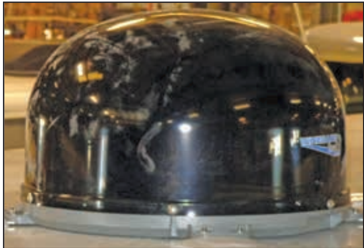
Figure 5-2: The dome satellite on top of the motorhome can be raised allowing easy access to change switches to a new satellite provider.
