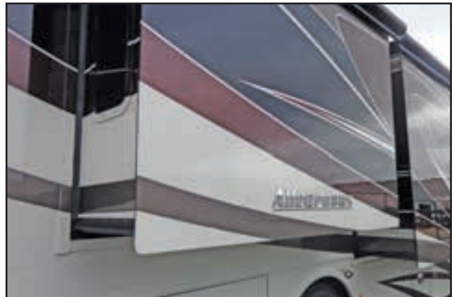
Figure 9-3: Typical slide-out fully extended
