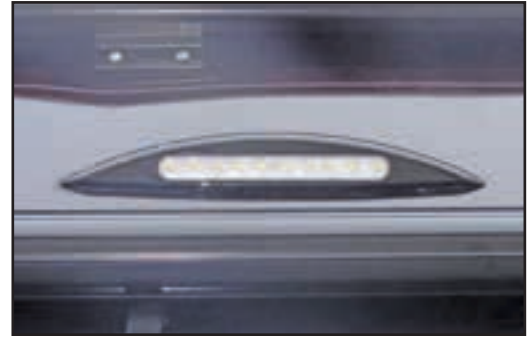
Figure 10-3: Exterior security light
