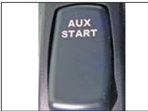
Figure 8-2: Auxiliary start switch
