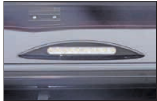
Figure 10-3: Exterior security light
