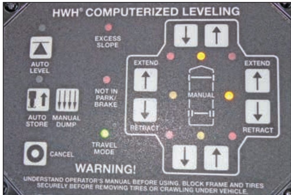
Figure 15-5: Leveling system control panel
