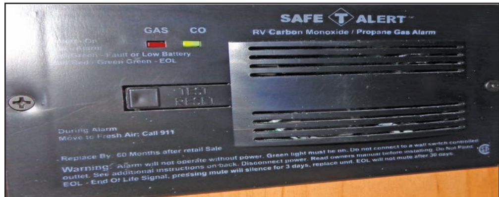
Figure 2-6: Carbon Monoxide alarm
