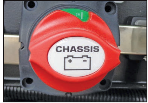
Figure 8-5: Engine battery disconnect panel switch
