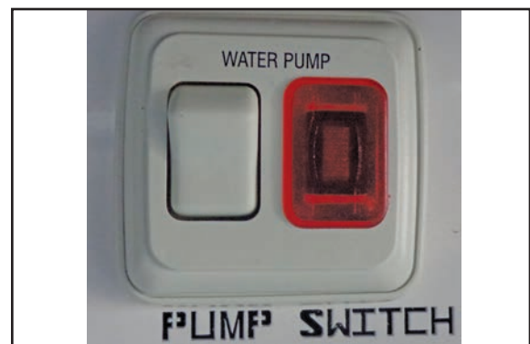
Figure 12-5: Water pump switch
