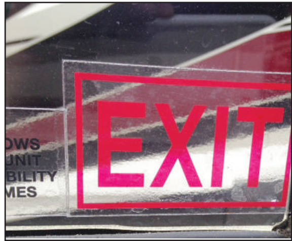
Figure 2-9: Emergency exit window
