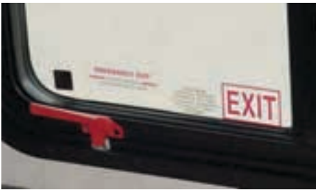
Figure 12-1. Emergency Exit Windows
