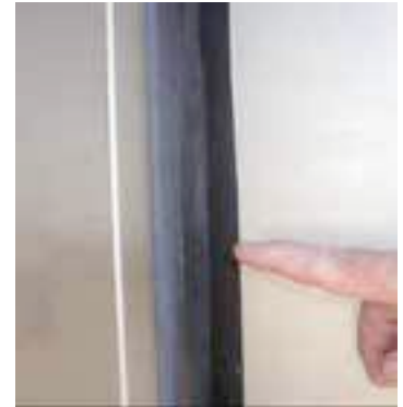
Figure 13-6. Inspecting Slide Out Gasket
