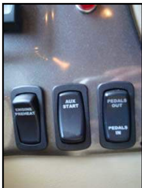
Figure 7-3. Auxiliary Start Switch (Center)
