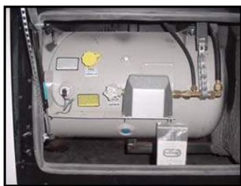
Figure 3-7 Liquid Propane Tank
