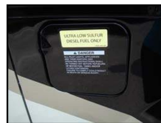
Figure 2-2. Fuel Tank Fill Door
