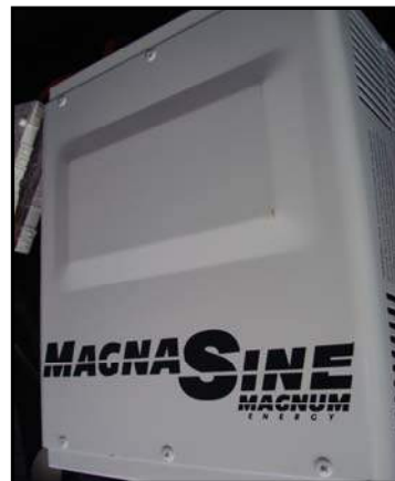
Figure 7-15. Sine Wave Inverter
