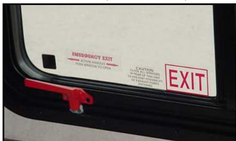
Figure 12-1. Emergency Exit Window
