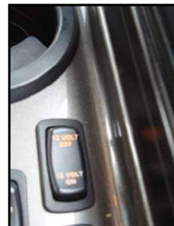
Figure 7-10. 12 VDC Disconnect Switch
