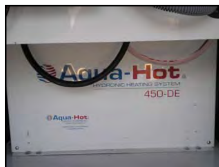
Figure 11-16. Hydronic Heating System
