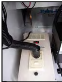
Figure 13-10. Vacuum Cleaner System
