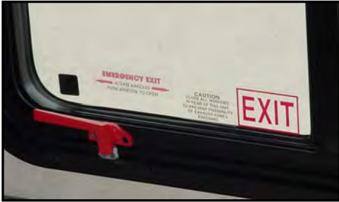
Figure 12-1. Emergency Exit Window
