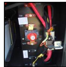
Figure 7-9. Rotary Switch to Disconnect “House” Batteries
