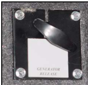
Figure 7-17. “Pull” Cable for Generator Release
