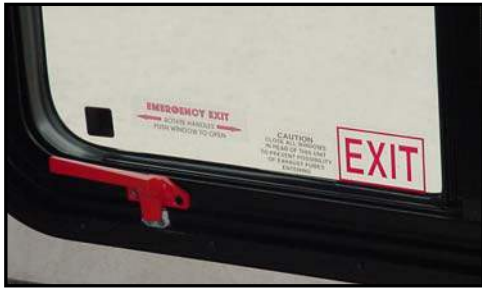
Figure 13-1. Emergency Exit Window
