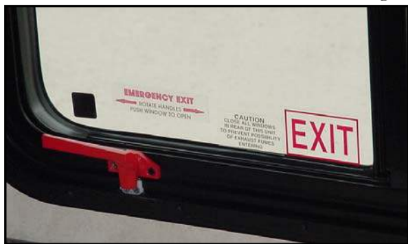
Figure 2-7. Emergency Exit Window
