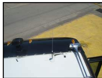
Figure 4-22. CB Antenna Installation
