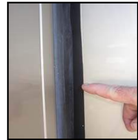
Figure 14-6. Inspecting Slide Out Gasket
