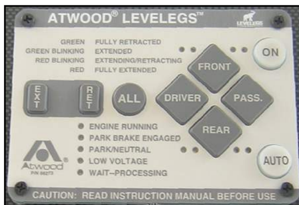
Figure 9-6. Leveling Control Panel on Dashboard
