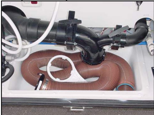
Figure 11-14. Sewer Hose and Drain Connections
