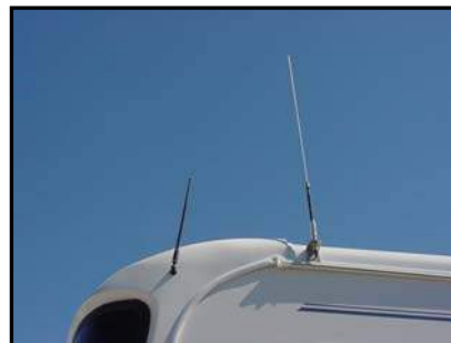
Figure 4-21. CB Antenna Installation
