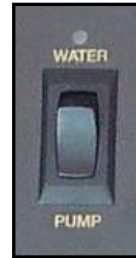
Fig. 11-5. Water Pump Switch
