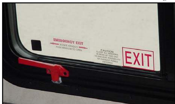
Figure 2-8. Emergency Exit Window
