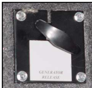
Figure 7-15. “Pull” Cable for Generator Release
