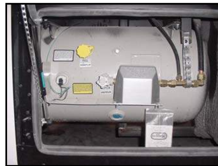
Figure 2-5. Liquid Propane Tank
