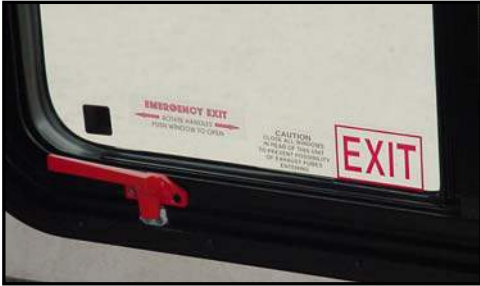
Figure 13-1. Emergency Exit Window
