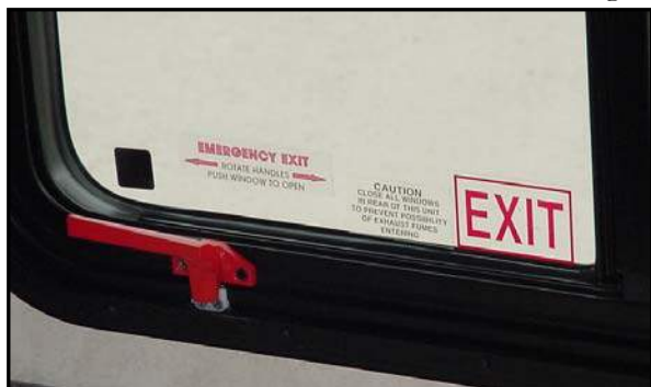
Figure 2-7. Emergency Exit Window
