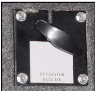
Figure 7-17. “Pull” Cable for Generator Release
