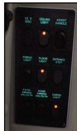
Figure 7-8. 12 VDC Disconnect Switch
