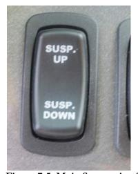
Figure 7-5: Main Suspension Switch
