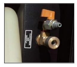
Figure 8-2: Rear Customer Air Supply
