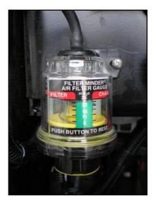
Figure 6-1: Filter Restriction Indicator
