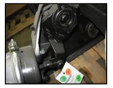
Figure 3-2: Automatic Slack Adjuster
