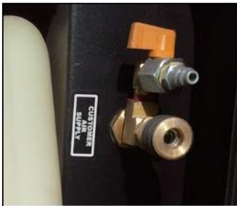
Figure 8-2: Rear Customer Air Supply
