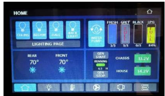
Figure 3-1: Spyder Controls System
