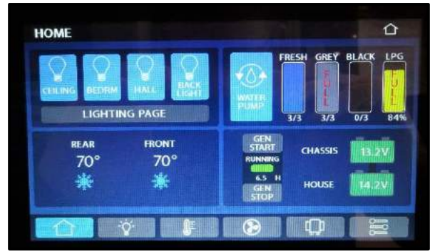
Figure 9-1: Spyder Controls System
