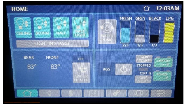
Figure 9-1: Spyder Controls System
