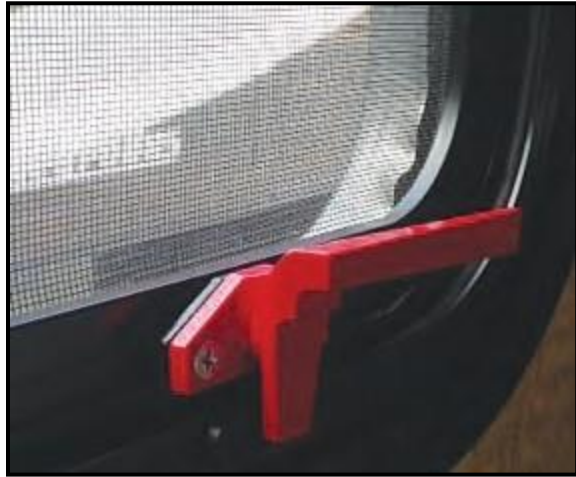
Figure 2-9: Emergency Exit Latch
