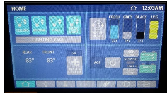
Figure 3-1: Spyder Controls System
