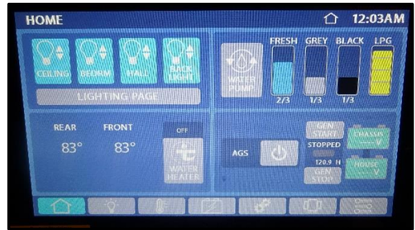
Figure 9-1: Spyder Controls System
