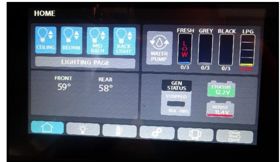
Figure 3-1: Spyder Controls System
