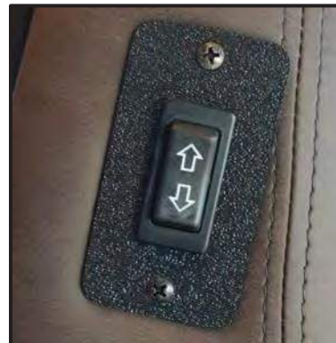
Figure 10-2: Front Slide-Out Switch
