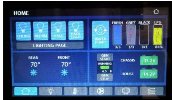
Figure 9-1: Spyder Controls System
