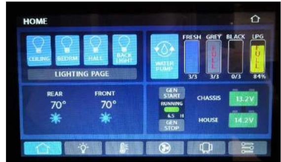
Figure 3-1: Spyder Controls System
