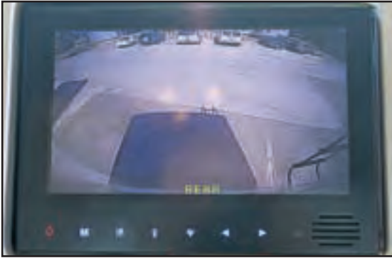
Figure 15-1: Rear-view camera monitor system
