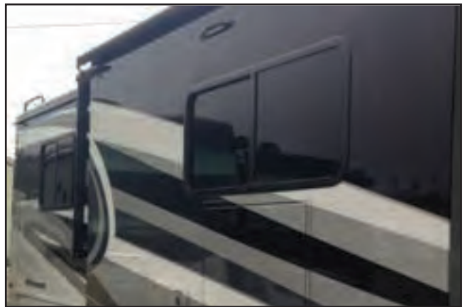
Figure 10-2: Typical slide-out fully extended
