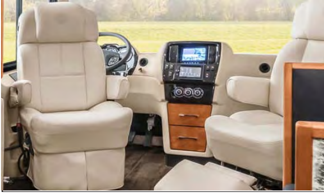
Figure 7-4: Both the driver and passenger chairs swivel to face the living area of the coach
