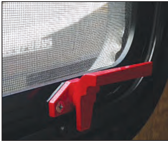
Figure 2-10: Emergency exit latch
