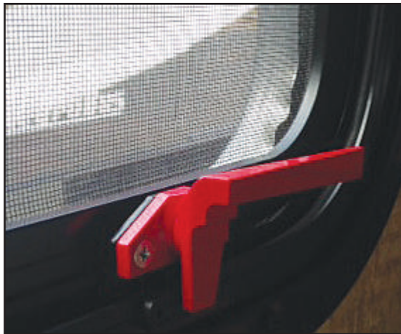
Figure 2-10: Emergency exit latch
