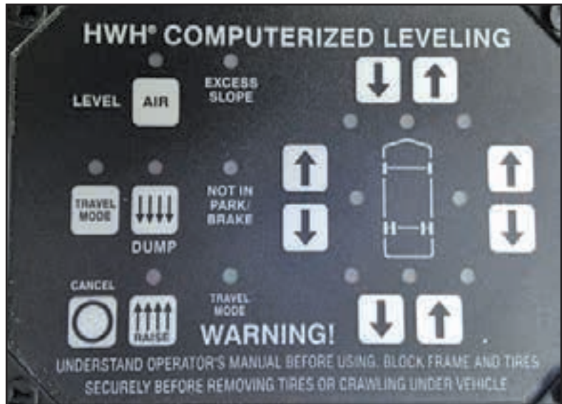
Figure 15-7: Leveling system control panel
