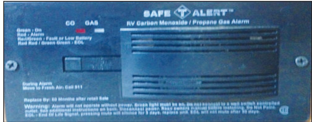
Figure 2-6: Carbon Monoxide alarm
