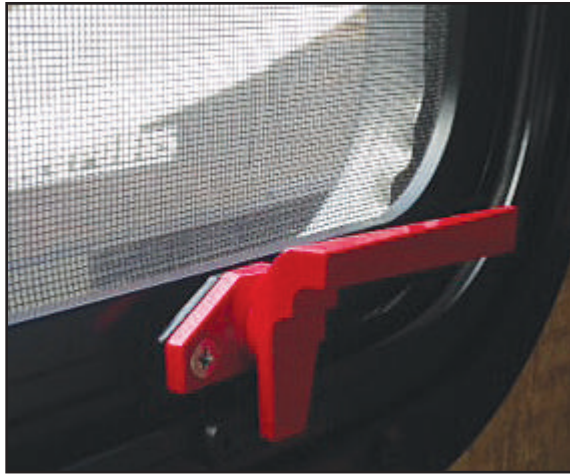
Figure 2-10: Emergency exit latch
