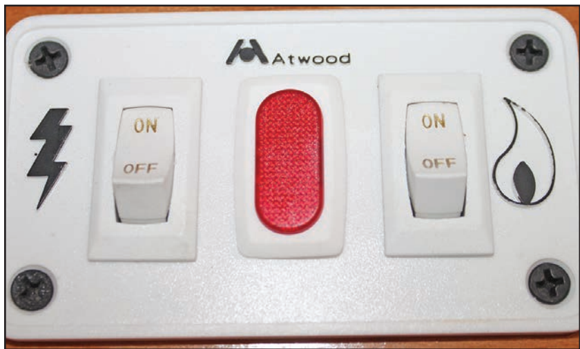
Figure 5-8: Water heater switches
