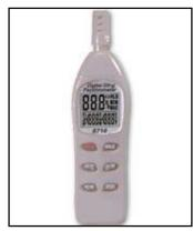
Figure 13-4. Portable Hygrometer
