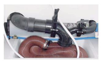
Figure 11-11. Sanitation Coupling, Valve and Hose
