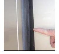
Figure 13-6. Inspecting Slide Out Gasket
