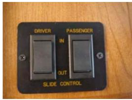
Figure 8-1. Slide-Out Switches
