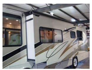
Figure 8-2. Typical Allegro Bus Slide-Out
