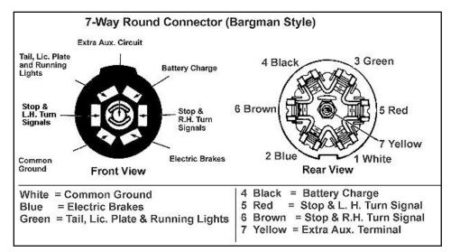
Figure 7-11. Seven-Pin Towing Connector
