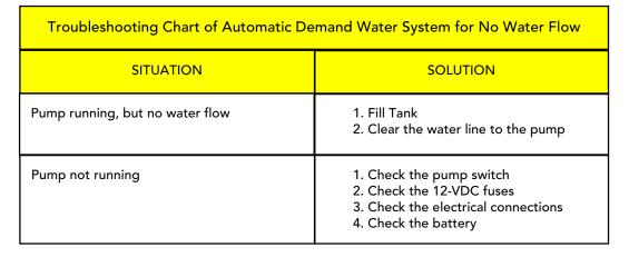
All of the water should be drained from the freshwater system when the unit is not in use for extended periods. For more detailed information regarding the water pump, one should refer to the water pump manufacturer's brochure in your Allegro Breeze Owner's Information Package.
