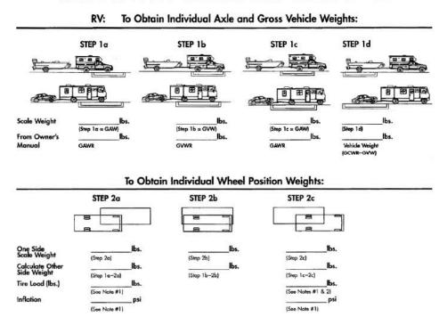
Figure 13-7. Procedure for Weighing the Motor Home (Each Tire Position Individually)
