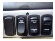
Figure 7-2. Auxiliary Start Switch
