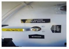
Figure 11-9. Water Heater Bypass System
