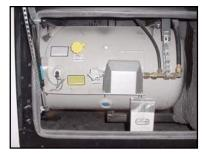
Figure 2-3. Liquid Propane Tank
