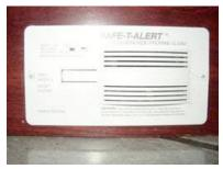
Figure 3-6. CO/LP Gas Detector
