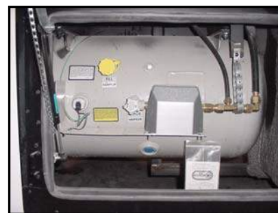
Figure 3-4. Liquid Propane Tank
