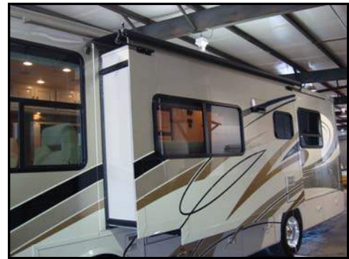
Figure 8-2. Typical Slide-Out Fully Extended
