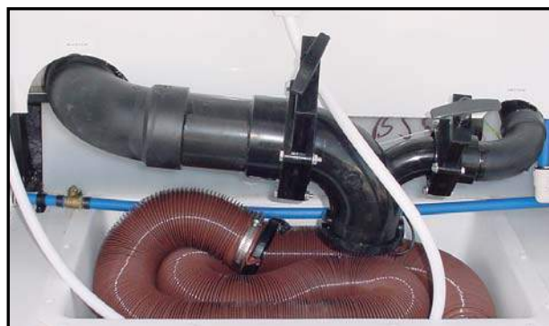
Figure 11-11. Sanitation Coupling, Valve, and Hose
