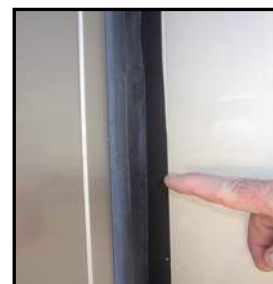
Figure 13-5. Inspecting Slide Out Gasket
