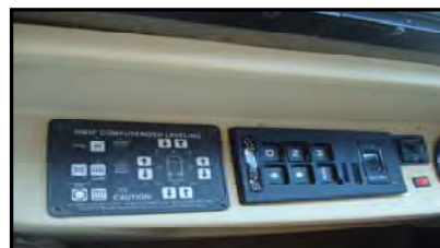
Figure 7-3. Driver's Side Console
