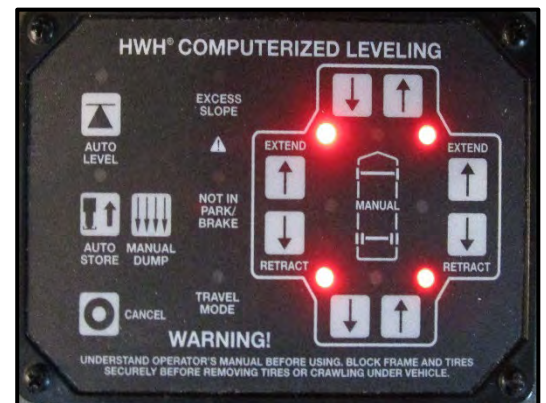
Figure 15-7 HWH Control Panel
