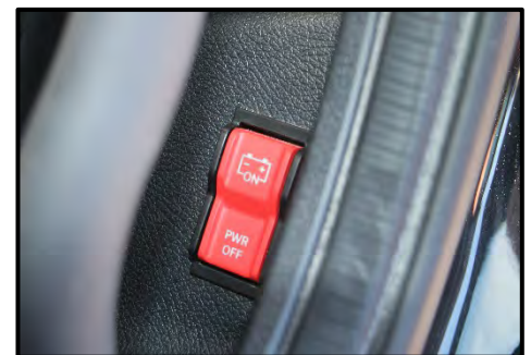
Figure 9-16 Engine Battery Switch
