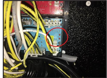
Figure 10-3: Location of Slide-Out Room Control Override
