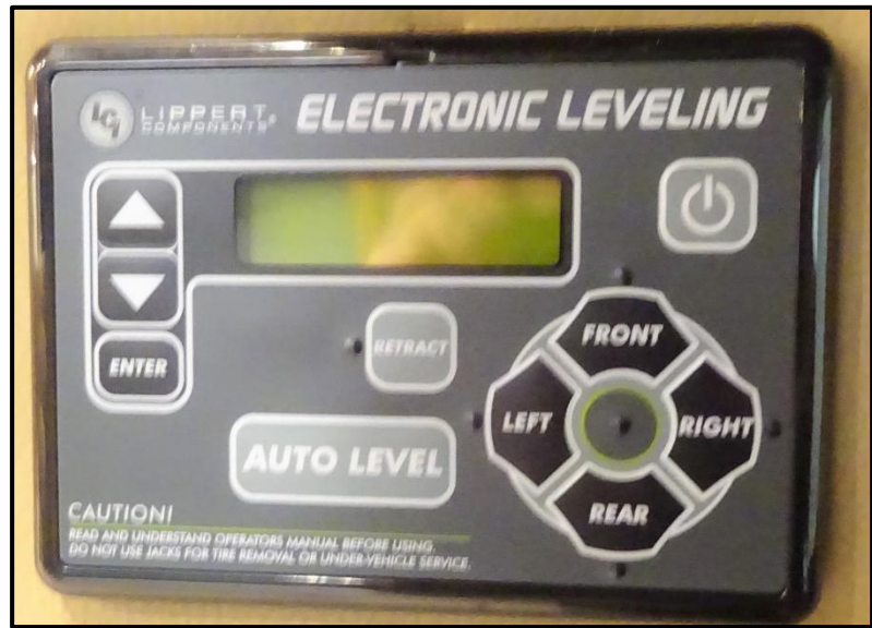
Figure 15-4: Leveling System Control Panel
