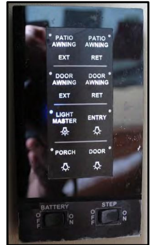
Figure 9-15: 12 VDC Disconnect Switch
