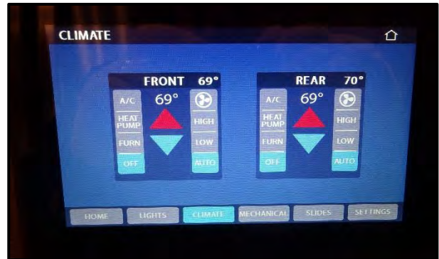
Figure 3-1: Spyder Controls System
