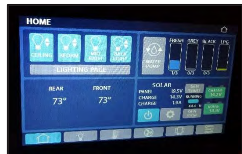
Figure 13-5: Spider Controls System Switch
