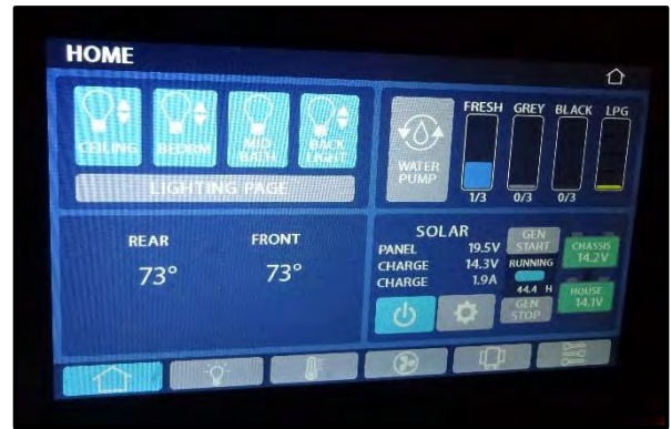
Figure 9-1: Spyder Controls System
