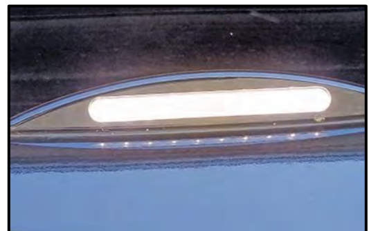
Figure 11-3: Exterior Security Light
