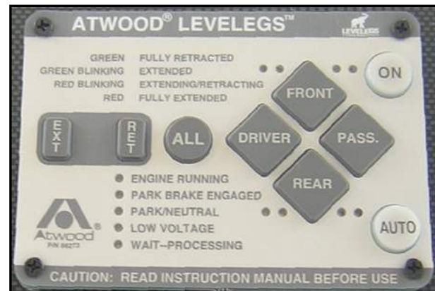
Figure 9-5. Leveling Control Panel on Dashboard
