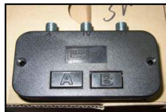
Figure 4-10. A/B Switcher Box for Tri-Pod Hookup
