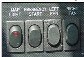
Figure 7-2. Auxiliary (Emergency) Start Switch
