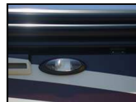
Figure 9-3. Security Light on Exterior
