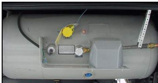
Figure 2-3. Liquid Propane Tank
