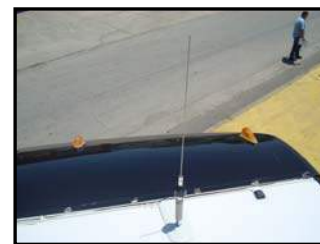
Figure 4-17. CB Antenna System
