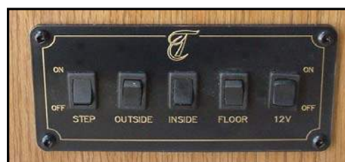
Figure 9-6. Electric Steps Switch (on left)
