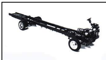
Figure 6-1. Typical Motor Home Chassis
