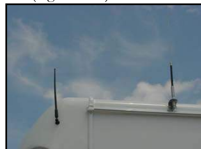
Figure 4-18. CB Antenna System
