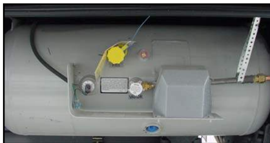
Figure 3-4. Liquid Propane Tank
