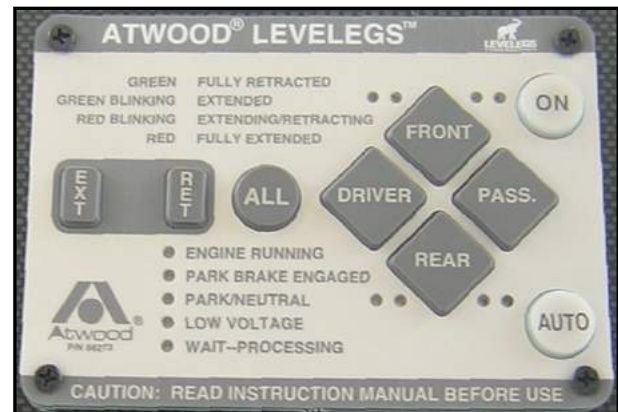
Figure 9-5. Leveling Control Panel on Dashboard
