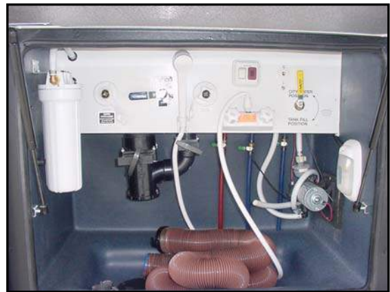
Figure 11-9. Sanitation Compartment with Wastewater Disposal Connection (Black Valve) and Wastewater Hose (Brown Hose)
