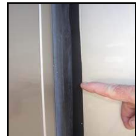
Figure 14-5. Inspecting Slide Out Gasket
