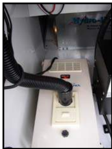
Figure 14-10. Vacuum Cleaner System
