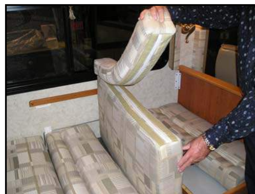
Figure 5-5. Filler Strip Attached to the Seat Portion
