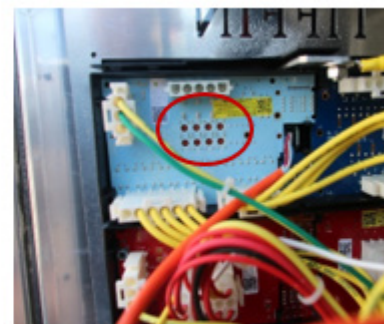
Step 5: Insert a round dowel in the control buttons to operate the Slide-Out Room.
