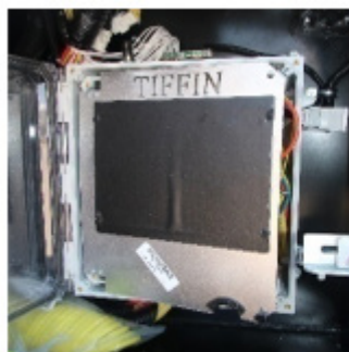
Step 3: With Thumb screws removed, Access M1 Circuit Panel.
