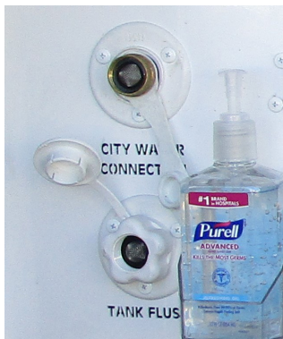
Fig. 13-15: Tank Flush Connection
