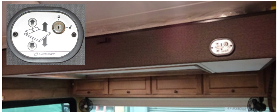
Fig. 12- 7 Overhead Drop Down Bunk Bed and Key Control Panel
