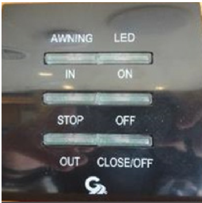
Fig. 14-1: Patio Awning Control Panel
