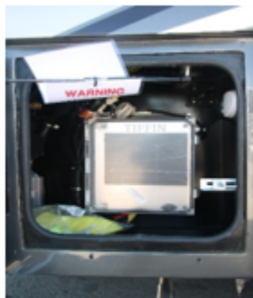
Figure 10-4: M1 Spyder Enclosure located in the driver's side exterior compartment.
