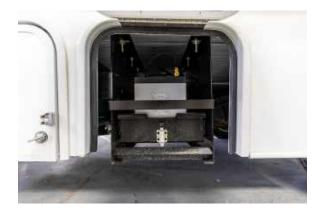
Image 57.1 Coach Battery Located in Drivers Side Compartment
