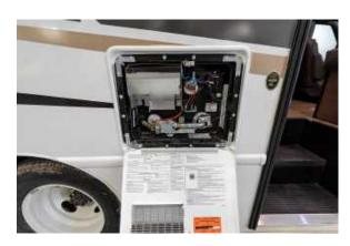
Image 83.1 Water Heater Exterior with Cover Opened
