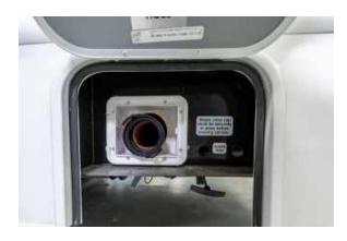
Image 89.1 Wastewater Dump Hose and Gate Valves
