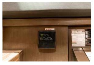
Image 73.1 Liquid Propane (LP) Gas/CO Detector
