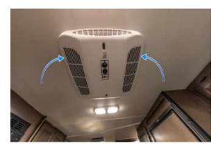
Image 69.1 Roof Air Conditioner with Air Vents Highlighted By Blue Arrows
