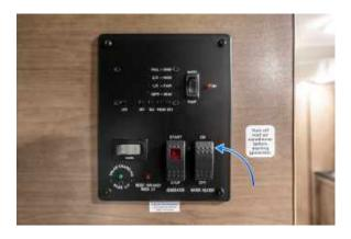
Image 82.1 Water Heater Switch On Monitor Panel
