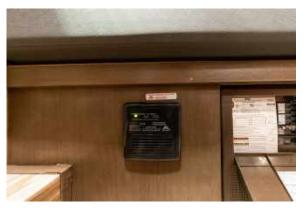
Image 46.1 Carbon Monoxide/Liquid Propane Detector Located In The Dinette Area
