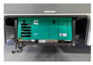
Image 63.1 Generator Located On Drivers Side of Motorhome
