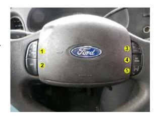
Image 22.1 Steering Wheel Cruise Control Buttons
