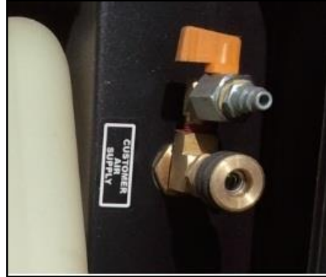
Figure 8-2: Rear Customer Air Supply
