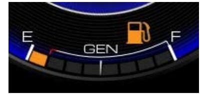
Fuel level low – generator will run out of fuel
