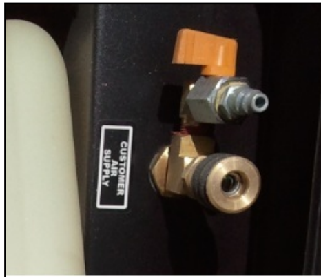
Figure 8-2: Rear Customer Air Supply
