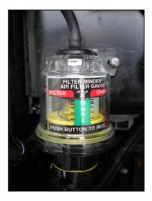
Figure 4-1: Filter Restriction Indicator
