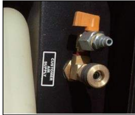
Figure 8-2: Rear Customer Air Supply
