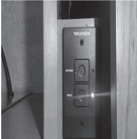
Figure: 6-2 Cable And Antenna Booster
