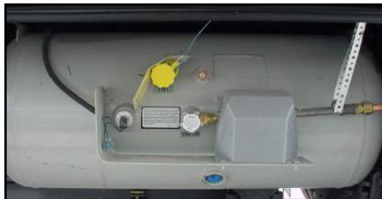
Figure 3-3. Liquid Propane Tank
