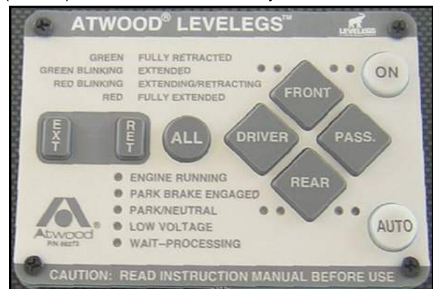
Figure 9-4. Leveling Control Panel on Dashboard
