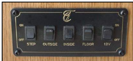
Figure 7-4. Battery Disconnect Panel
