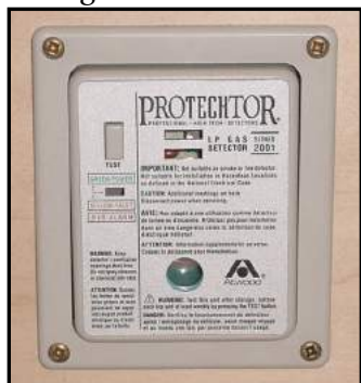
Figure 3-4. Propane Gas Detector
