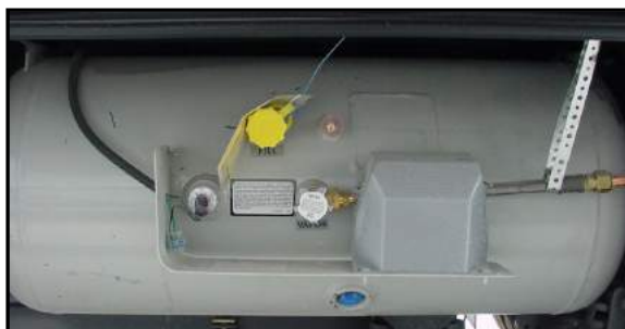
Figure 2-4. Liquid Propane Tank
