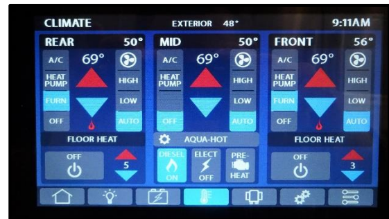
Figure 4-3: Spyder Controls System
