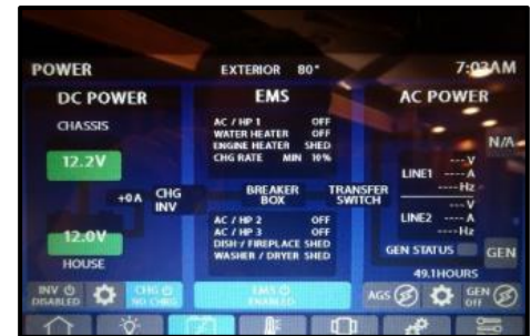
Figure 10-13: Energy Management System
