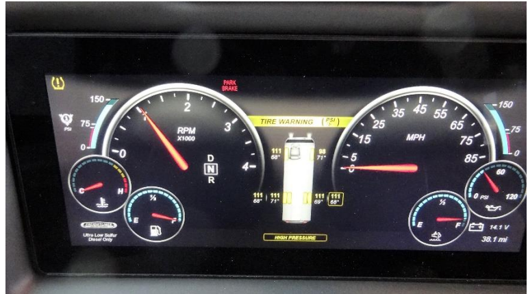
Figure 16:4 Instrument Panel Tire Pressure Monitor
