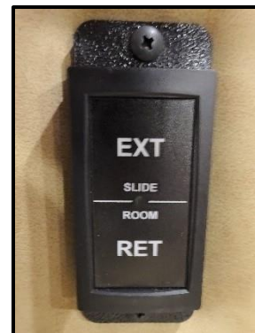
Figure 10-2: Front Slide-Out Switch
